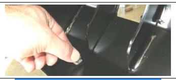
47. Fit 4 x M6 cage nuts to bottom inside face of lower pan in square holes as shown.
