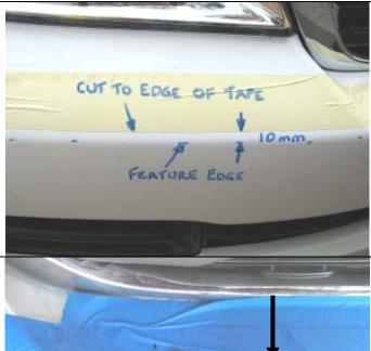
Apply wide masking tape edge, carefully aligning 10mm above bumper feature line as shown. Keep the same line level through the centre section of the bumper as shown
