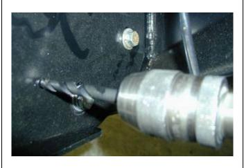
65. With access through light aperture in wing, using the M10 pilot holes in mount brackets (located up 175mm from bottom face of bar), drill pinning hole through uprights on bull bar. Fit M10 screw, washer set and flange nut and do up tight.
