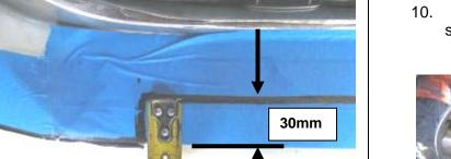
Mark out centre cut area of bumper as shown, 740mm wide x 30mm back from feature edge.
