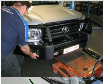
59. With the aid of a lift table or one or more assistants carefully and safely lift, position and bolt the bull bar to the mounts using 6 x M12 bolts, large flat washers and spring washers. Centralise the bar to the front of the vehicle and adjust height.
