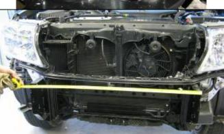
58. Tap the outer flange of the mount brackets until they are hard up against the tow hook mount area. Nip up the lowest outboard nut on each bracket. Brackets should be about 935mm apart
