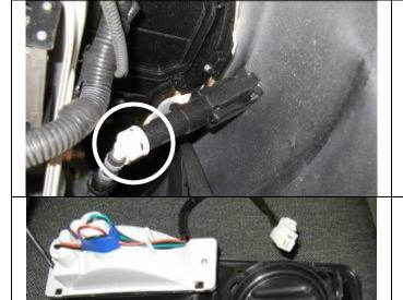
66. If headlight cleaner system to be fitted, reconnect circuit at main joint to vehicle and also hoses to tails of spray heads
