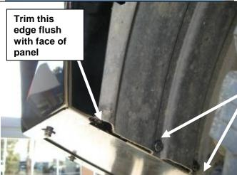
82. Fit 5 x M6 cage nuts to each wing splash panel as shown on *inside* faces.
