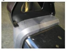
Adjust buffers so they sit neatly on the bull bar profile then secure using M6 flange nuts over studs.
