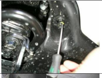
When removing lower trim panels, a plastic nut located on each side will need to be prized open with a small flat blade screwdriver to assist removal.
