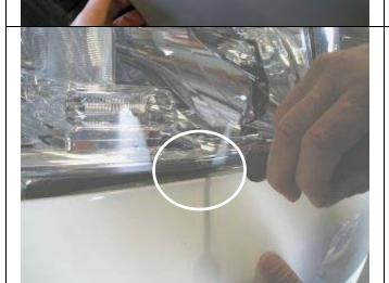
21. Push bumper down immediately below headlamp to gain access with a small flat blade screwdriver and release holding tab.
