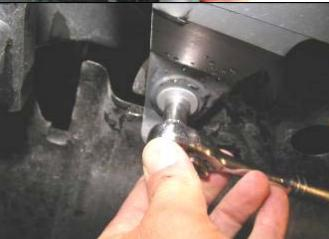
6. Remove lower bumper retaining screws.
