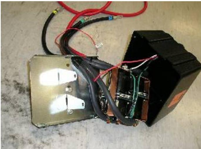
1. Remove the four solenoids from the base of the control box using the copper bus bar as an aid and hold to one side.
