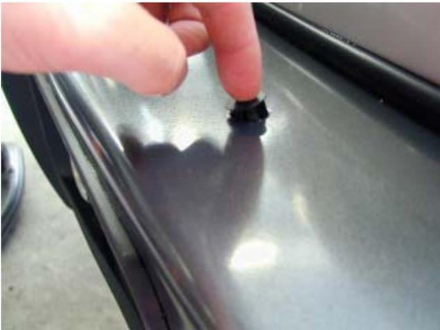
If fitted, headlight washers can be mounted through the Diameter 22 holes on the top face of the wing. Assemble using the existing mount clips. Two plugs are provided to cover the holes if there are no headlight washers on the vehicle.
