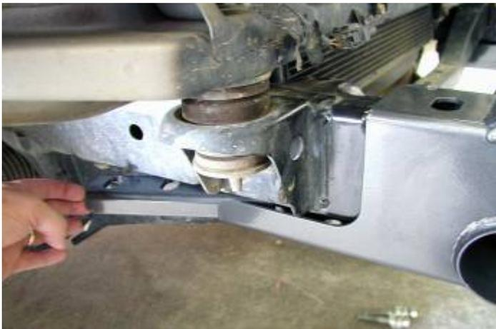
1. Slide the mount assy. over the chassis rails. Try not to shake the vehicle too severely as the tube packers may fall out of place.
