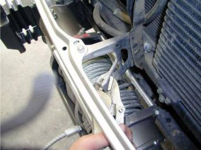
1. Using vice grips, multi grips or pliers bend back the bumper mounting arm approximately 30 – 40 degree's to clear bar when assembled.
