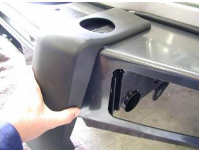
1. Fit the buffers. Buffer studs fit through the slots in the wings and the pan. Fasten using M6 flange nuts.
