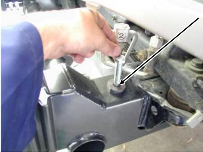
1. Insert the M12 X 200mm bolt through the top hole using one of the 10mm thick packers. Push through while removing the screwdriver from underneath until the bolt locates right through
