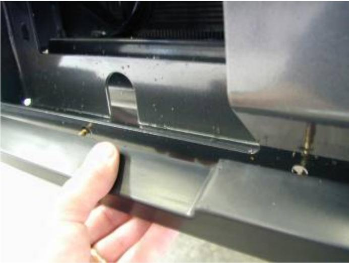
1. Position the lower buffer on the winch bumper and assemble using the M6 flange nuts.
