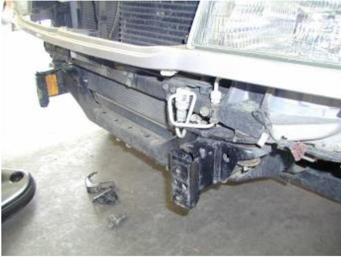
1. Disassemble the mount assy. from the winch bumper by removing the transit bolts.
