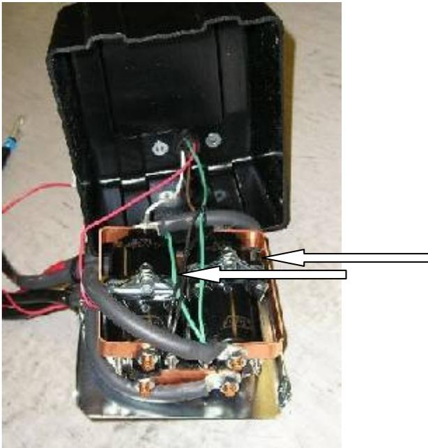
1. Remove the two cap screws, nuts and spacer washers that hold the four solenoids in place.
