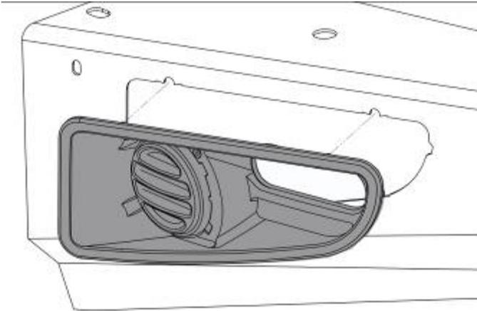
Assemble and install combination light surrounds (p/n 3163015) as per instructions no. 3786421 supplied with surround kit. Note: Optional fog lamps can be installed at this point as per fitting instruction no. 3783315 supplied with fog lamp kit no. 6821201. Wire the combination lamp to the vehicles indicator and clearance lamps.
